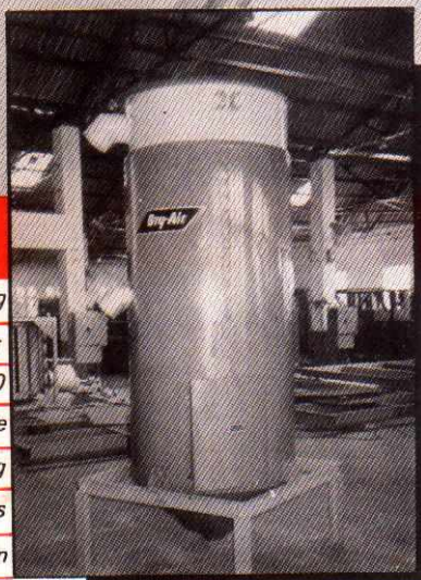
The Drying Hopper Model H 160 capable of handling 1600 lbs of plastic resin
