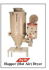
drying is faster. However, with heating, the dewpoint and moisture content remains unchanged. As a result, there is no positive removal of moisture from the environment. The moisture equilibrium content of the plastic pellet can be limited. Thus, the degree of dryness will also be limited. This is particularly true for all hygroscopic plastic resins. Hot air drying is recommended for non-hygroscopic resins where the moisture is present on the surface.
