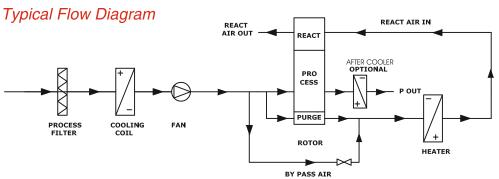
The heart of Bry-Air's Mould Dehumidification System is the Honey Comb Dessicant Wheel which ensures optimum results year round by simply lowering the dewpoint surrounding the moulds by approximately 5 to 10 degrees lower than the temperature of the chilled water in the mould. By
