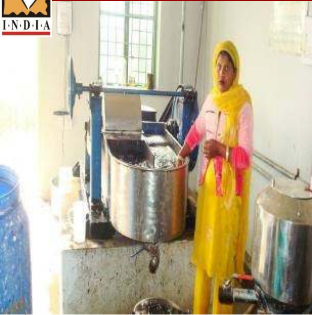
The Beater which performs the first leg, where water, shredded paper and cloth strips are beaten into pulp. ↓
