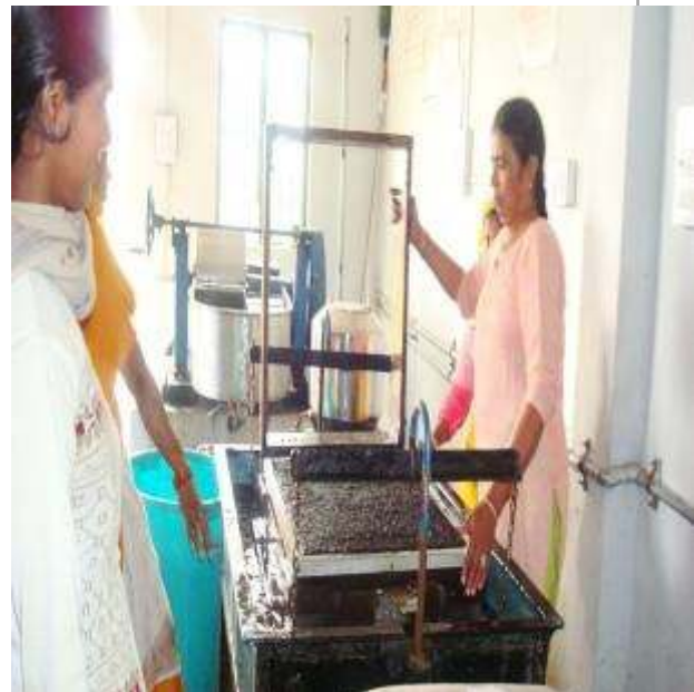
The pulp is taken out in the form of a sheet
