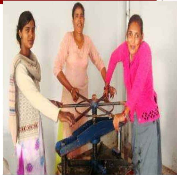
Sheet is then pressed to squeeze out the water ↑
