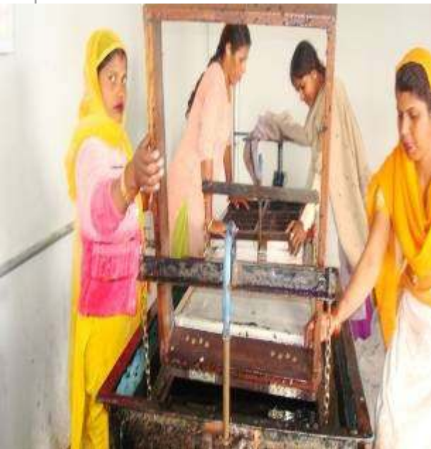
The pulp is then spread onto the frame →
