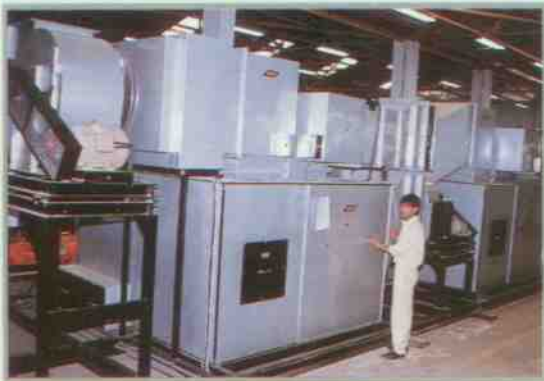
Engineered Dehumidifier MVB75E for bagging of Caustic soda.
