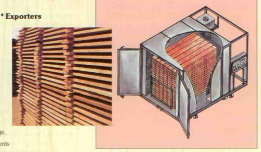
The Bry Air Dehumidifier 'built-in' system increases the vapor pressure difference removing moisture from the air surrounding the 'wet' wood in the chamber. The moist air is drawn into the dehumidifier where the moisture is adsorbed by a rotating desiccant bed and ducted out. The now, dry air flows back into the chamber increasing the vapor pressure difference and thus forcing the wood to give up it's moisture to the dry surrounding air.
